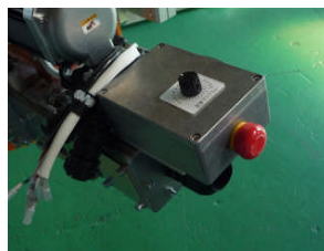
Selector switch box for welding conditions
